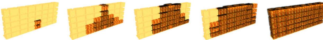
Figure 2: Simulated fire spread in one storage rack unit in a cold storage.
