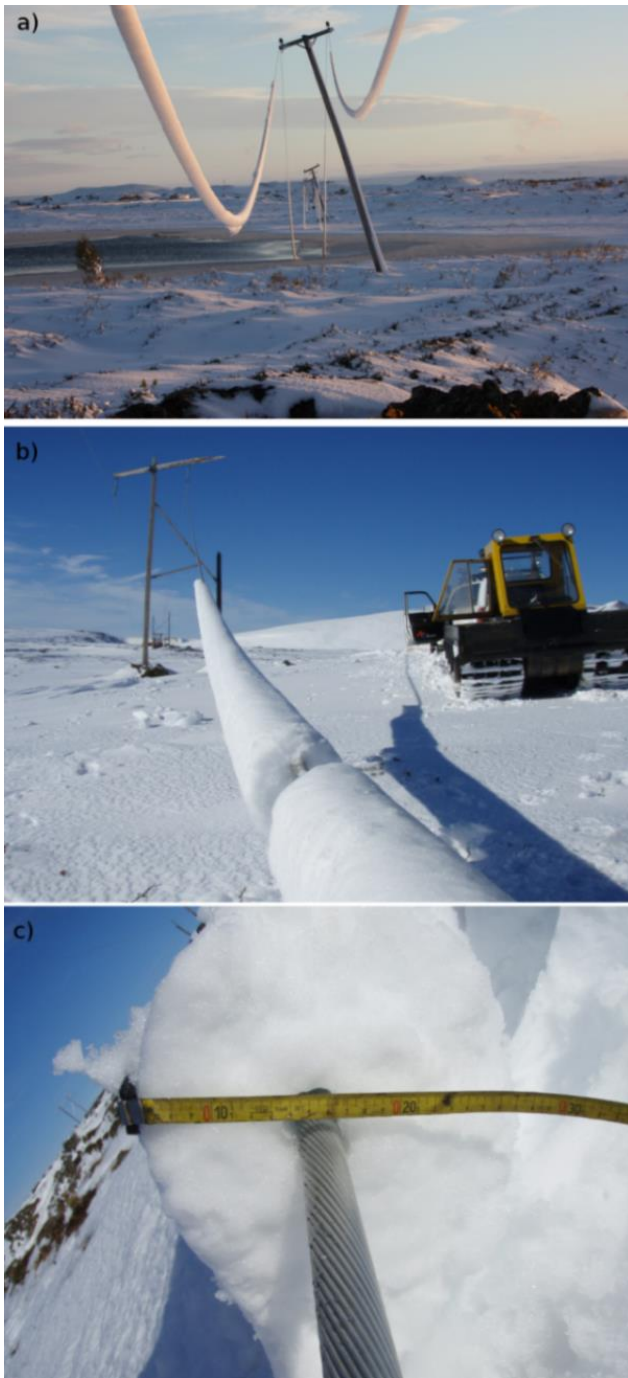
Fig. 6. Photos from the wet-snow event on 10 September in North Iceland. a) Loaded conductors and leaning poles of the distribution system north of Lake Mývatn. b) Accumulated wet snow and broken transmission towers in 132 kV KS1 at Reykjaheiði. c) Wet snow sample on a faulted transmission line conductor on Reykjaheiði, measuring 21 cm mid-span which is however not an average value for the area.
