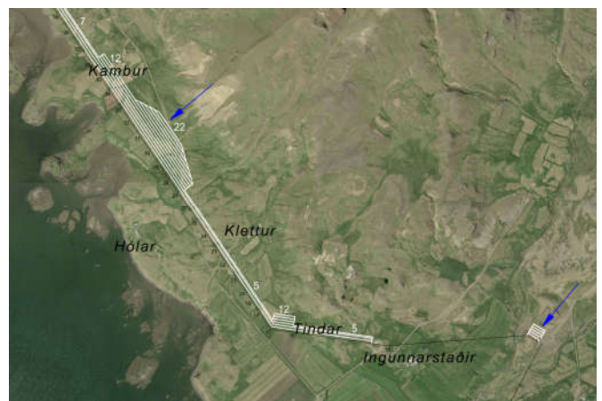
Fig. 6 Wet-snow icing on Mjólkárína 1, West Iceland, 20 February 2014. The icing diameter at each line section is shown.
